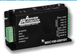
The MDC100-050101 driver is designed to drive DC Brushless motors at currents of up to 10A (peak) and 50V. Using hall sensor feedback, a constant velocity mode can be selected. The driver is protected against over current (cycle-by-cycle), hall sensor error and under voltage. When an error occurs, a fault light is turned on to notify the user.
